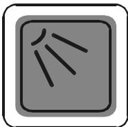
The programme button (6) is lit **red**: the boiler and tank are filling and heating up.
