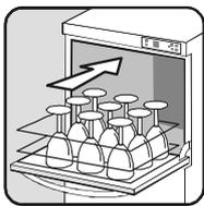
Push the full wash rack into the machine and close the door.
