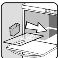
Reinsert the flat filter with the filter cartridge.
