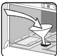
Open the screw cap on the salt container, insert the funnel into the filler opening and add three bags of Winterhalter special salt (= 1.5 kg).
